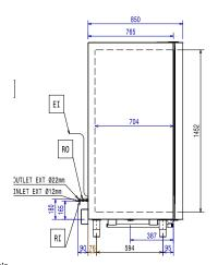
Drain Electrical inlet (power) RΩ Refrigerant Outlet
